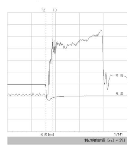
T2: Starting point of voltage drop when Power off
